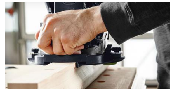
Trim Stop Achieve precise, repeatable mortises.
